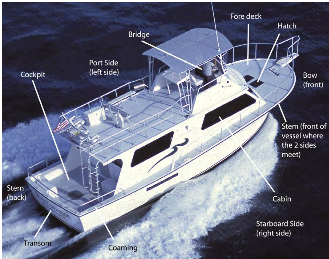
FIGURE 1-92 PARTS OF A HULL AND VESSEL
