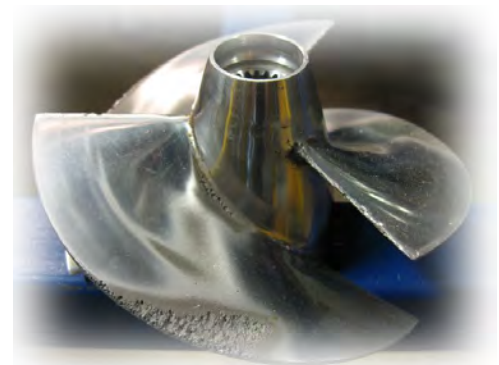
FIGURE 13-8 CORRODED PROP DUE TO CAVITATION
