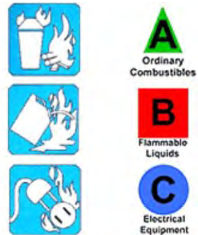
FIGURE 3-7 FIRE RATING SYSTEM
