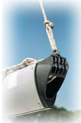
FIGURE 15-14 BOOM TOPPING LIFT
