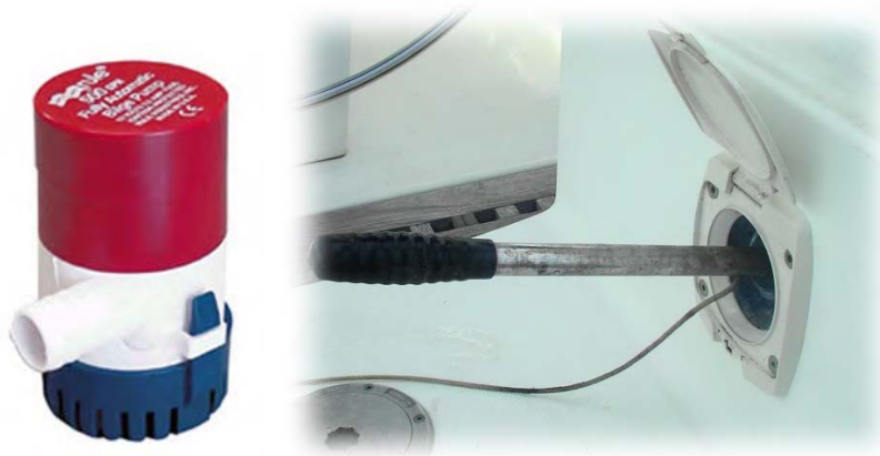
FIGURE 1-64 ELECTRIC &amp; MANUAL BILGE PUMPS
