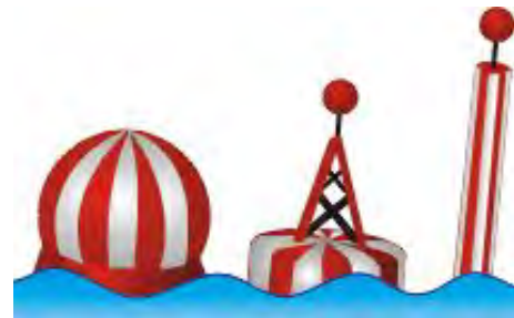
FIGURE 21-6 SAFE WATER MARK
